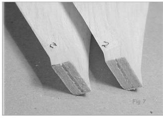
Fig. 7 Blades ready for insertion of new hub
