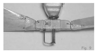
Fig. 9 Completed hub and blades of the folding propeller. Note kook on hub for small rubber band to close low blade when folded.
