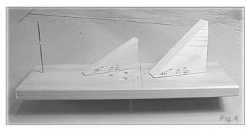
Fig. 4 Fixture for drilling hinge angles and setting proper pitch
