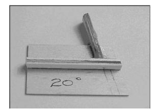
Fig. 2 Top view of the 20 deg. compound angle jig
